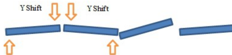
Img. 3.6.3-1 Y-correction shifting point
